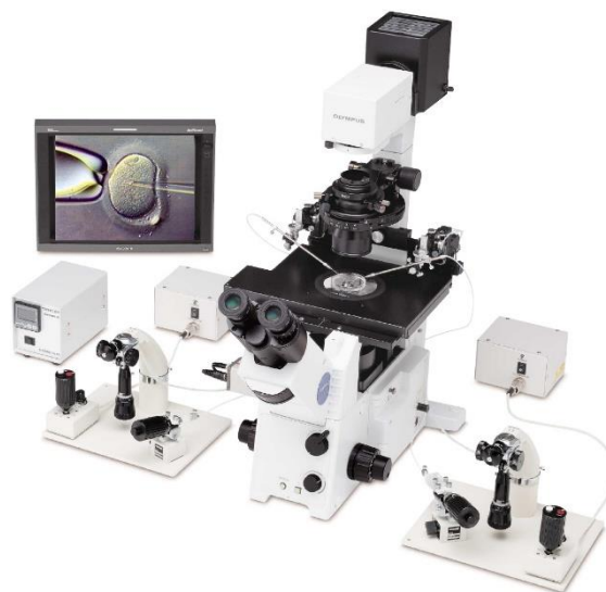
Fig. 4. An automated system for microsurgery of the cell, including an inverted microscope, motorized micro-tool holders, micro-pumps and a video monitoring device
